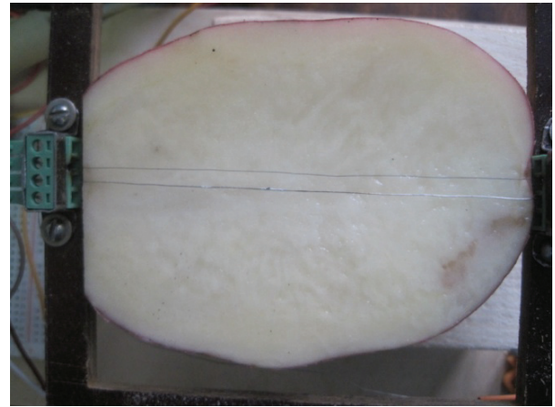
Fig. 7. Placing a thermocouple and heater on the potato tuber plant tissue
