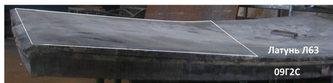
Fig. 1. The view of bimetallic sheet after explosion welding
