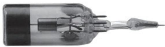
Fig. 4. Cathodoluminescent lamp of a triode structure
