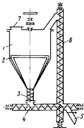
Fig. 1. A design of filling-type mixer
