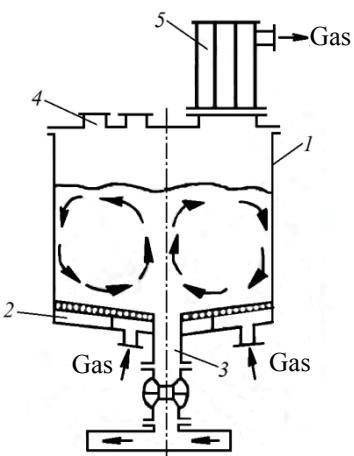
Fig. 4. Design of pneumatic homogenizer
