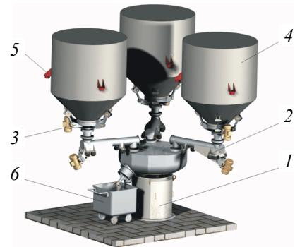
Fig. 9. UMKS-1.0 technological system for multi-component mixing of bulk materials
