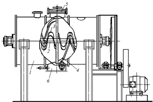
Fig. 5. Design of a drum mixer
