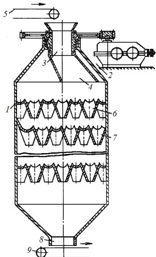
**Fig. 6. Design of a mixing device for bulk materials**
