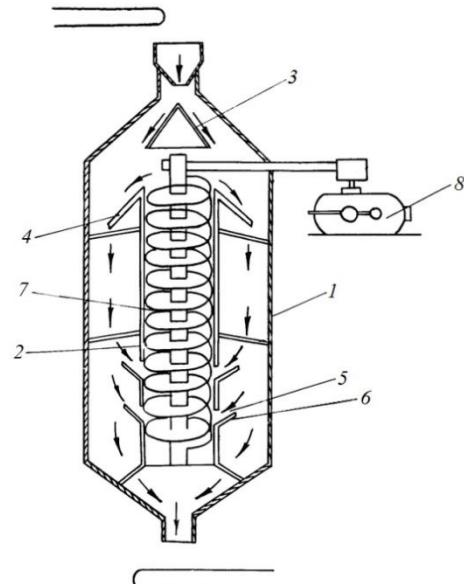
Fig. 8. Device for homogenization of bulk materials
