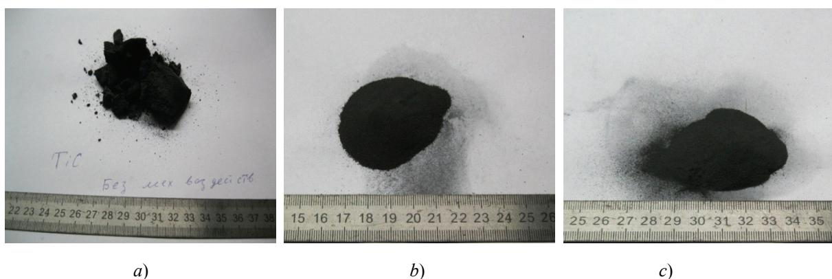
**Fig. 1. General view of synthesized titanium carbide powder produced by:**
