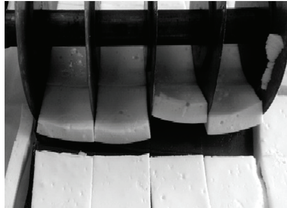
Fig. 6. Adhesion failure in forming combined bodies by smearing and cutting methods
