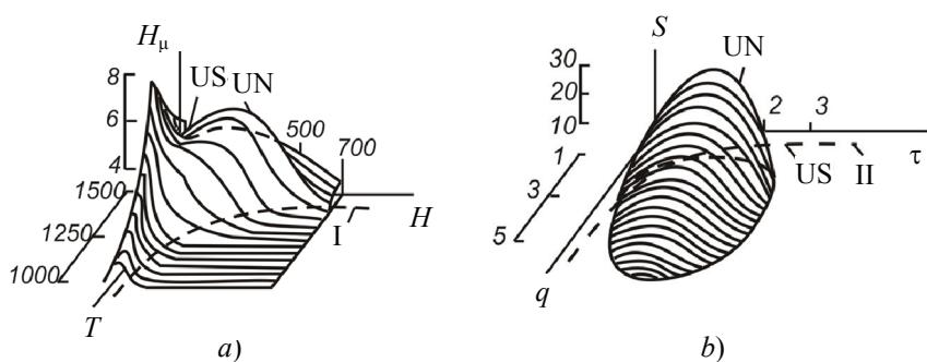
Fig. 1. Distribution of microhardness  $H_\mu$ , GPa along the depth  $H$ , μm of the surface layer of a titanium alloy with a chrome-nickel coating with a change in temperature  $T$ , K (a) and the relative surface area  $S$ , % with a modified structure depending on the specific power  $q$ , kW/cm<sup>2</sup> and duration  $\tau$ , s of the electron-beam heating (b); the visible boundary of the modified layer (I) and the melting boundary (II) are marked with dashed lines
