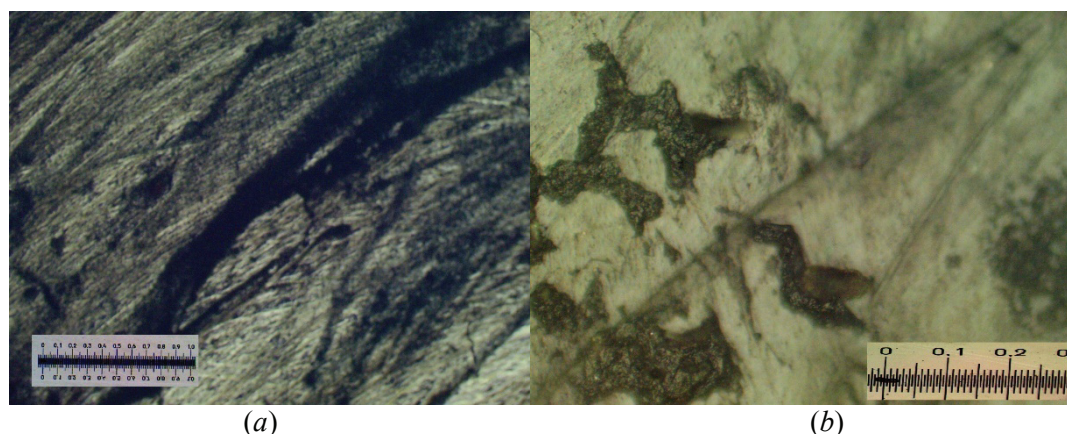
Fig. 2. Pressing surface from nanodiamonds modified with sp^2 -carbon: a - \times 100 ; b - \times 400
