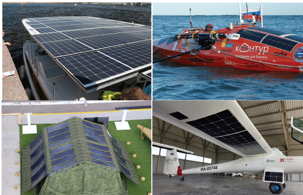
Fig. 1. Examples of completed projects for the integration of semi-flexible lightweight PVMs in sea, air, and mobile deployable applications
