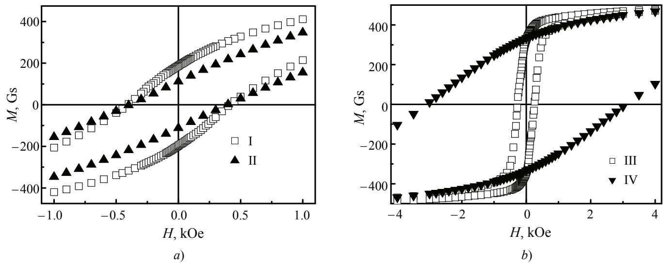
**Fig. 2. Dependence of magnetic moment for sample before and after annealing in free powder (I and III) and fixed in polymer matrix (II and IV) on external magnetic field at  $T = 300$  K:**
