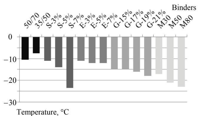
Fig. 9. The mean values of breaking point of bitumen binders produced in Poland
