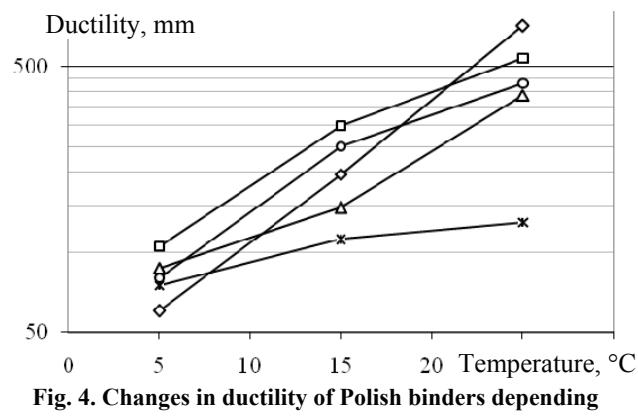
Fig. 4. Changes in ductility of Polish binders depending on the temperature:
