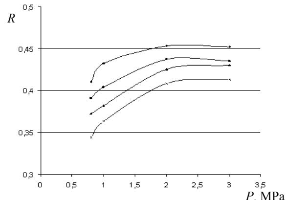
**Fig. 5. The dependence of UAM-150 membranes retention coefficient on the concentration of the feed solution and pressure; concentrations,  $\text{kg}/\text{m}^3$  are designated:**
