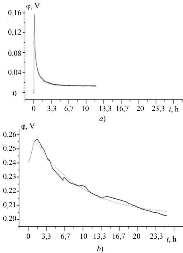
**Fig. 8. Dependence of the membrane potentials on the time in full osmosis:**
