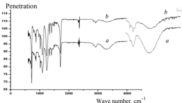
**Fig. 3. IR spectra of the diffuse reflection from the surface of the MGA-95 cellulose acetate polymer membrane:**
