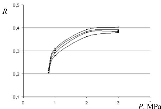
**Fig. 6. The dependence of UAM-150 membranes retention coefficient on the concentration of the feed solution and pressure; concentrations,  $\text{kg}/\text{m}^3$  are designated:  $C_1 = 4.27$ ;  $C_2 = 5.32$ ;  $C_3 = 6.24$ ;  $C_4 = 8.40$**
