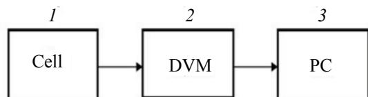
**Fig. 2. Diagram of the setup to study membrane potential:**
