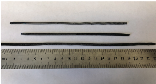
Fig. 1. TiB – 30 wt. % Ti rods obtained by SHS-extrusion
