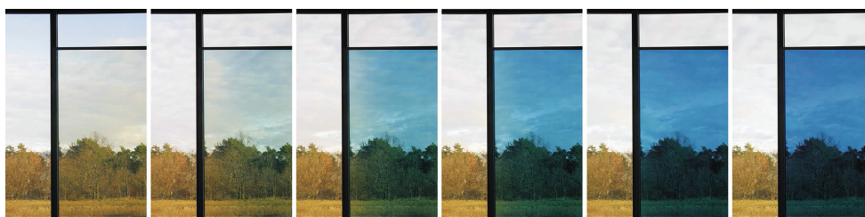
Fig. 10. Six different tint states of the Smart Window based on tungsten oxide and Prussian blue as electrochromic layers and PVB ion-conducting polymer electrolyte
