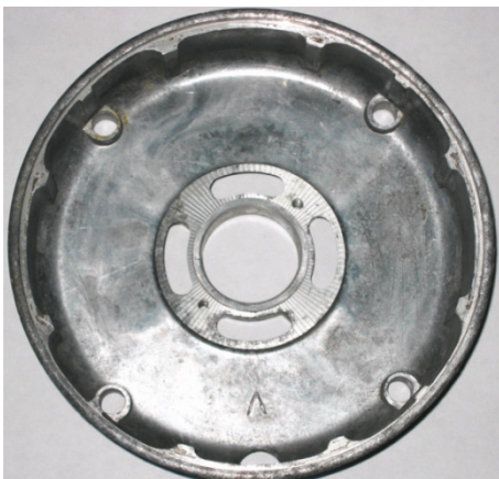
Fig. 1. General view of the end shield of the electric motor
