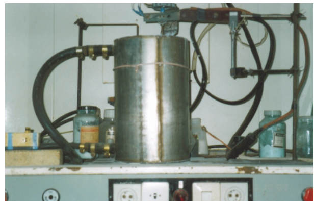
Fig. 3. General view of the laboratory setup for MAO: a – power supply and control unit; b – electrolytic bath
