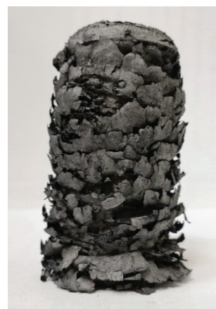
Fig. 2. Physical appearance of graphene-containing sorbent based on rapeseed
