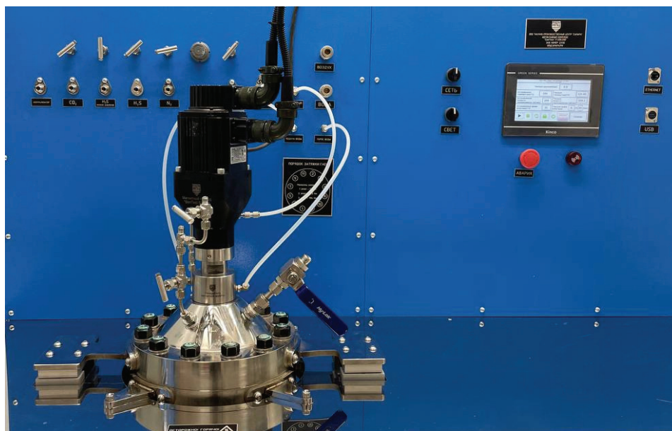
Fig. 4. Autoclave complex designed to simulate the operating conditions of tubular products during the extraction of petroleum fluid
